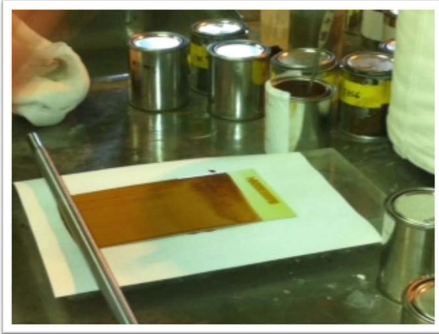
Paint is drawn down across the metal as uniformly as possible. The metal is then cured in a small oven and cut to size. This process limits the drawdown size to standard 3"x5"
