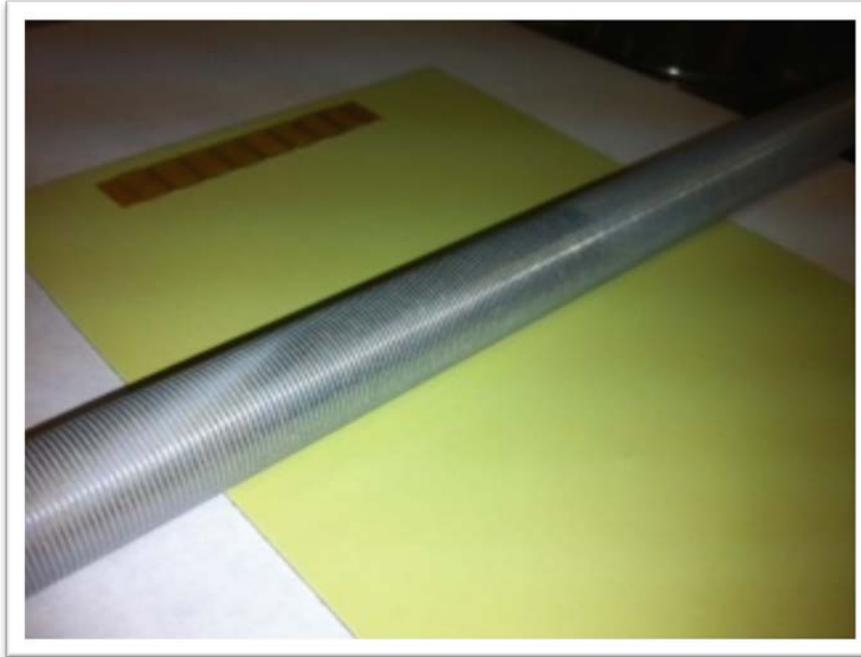
This is a close up view of the bar used to make the paint drawdown. With solid colors there are no lines visible in the paint. With Mica and Metallic colors however, the flakes orient directionally with the threading – giving the drawdown line appearance.
