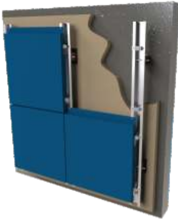
T-cassettes & LCH-1 Cassettes installation system
