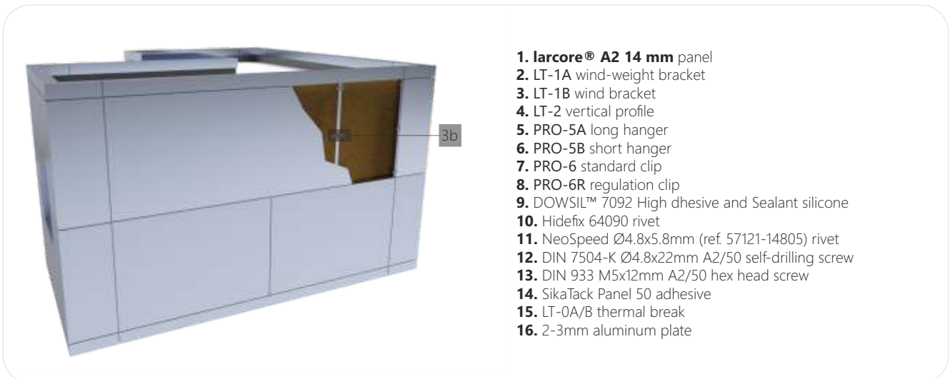
3b. Intermediate long hanger with bracket LT-1A/B 60-160
