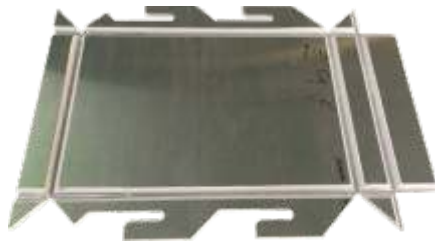
1. Cut and routing the panel according to the standard geometry.
